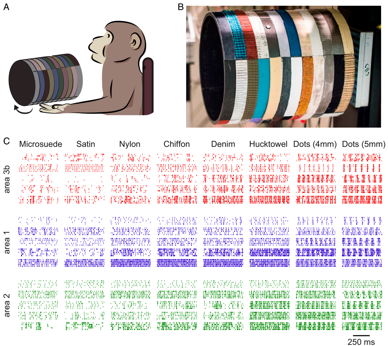
Fig. 1. Experimental apparatus and sample texture responses. (A) Textures were passively presented to the distal finger pads of awake macaques. (B) The rotating drum stimulator—on which the 59 textures were mounted—allows a surface to be scanned across the fingertip at a precise and repeatable speed and depth of indentation into the skin. (C) Sample spiking responses of five neurons each in areas 3b, 1, and 2 to five repetitions of eight textured surfaces.
